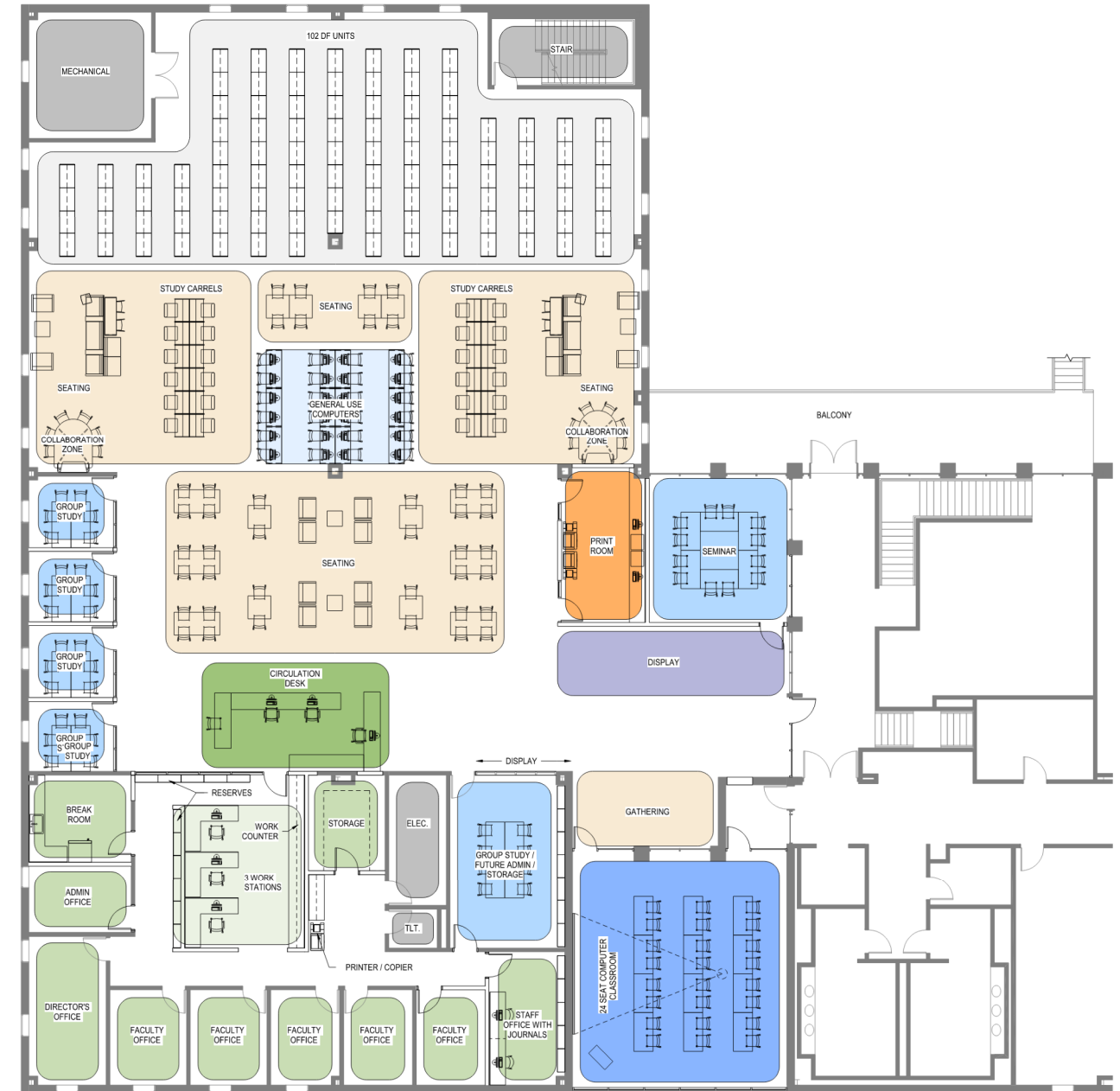
1B EXPANDED FOOTPRINT 11,156 SF of renovated space + 886 SF of new construction
